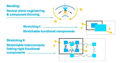
**Figure 3.2.-1.** Overview of fundamental strategies adopted to achieve flexibility and/or stretchability of sensors and electronic components as summarized by [7].
